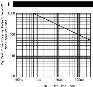
NOTE: This P<sub>PP</sub> versus time graph allows the designer to use these parts over a broad power spectrum using the guidelines illustrated in App Note 104 on Microsemi's website. Aircraft transients are described with exponential decaying waveforms. For suppression of squarewave impulses, derate power and current to 66% of that for exponential decay shown in Figure 1.
