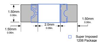
Recommended Soldering Pattern for reflow soldering of the BC (1206) package.
