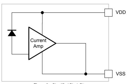
Figure 3 – Simplified Block Diagram
