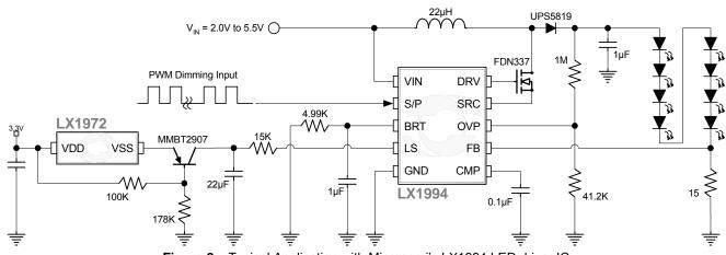
Figure 8 - Typical Application with Microsemi's LX1994 LED driver IC
