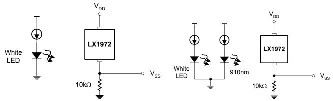
Figure 1 – Operational Voltage Measurement Circuit
