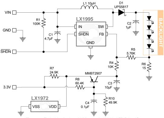
Figure 7 – Typical Application with Microsemi's LX1995 LED Driver IC
