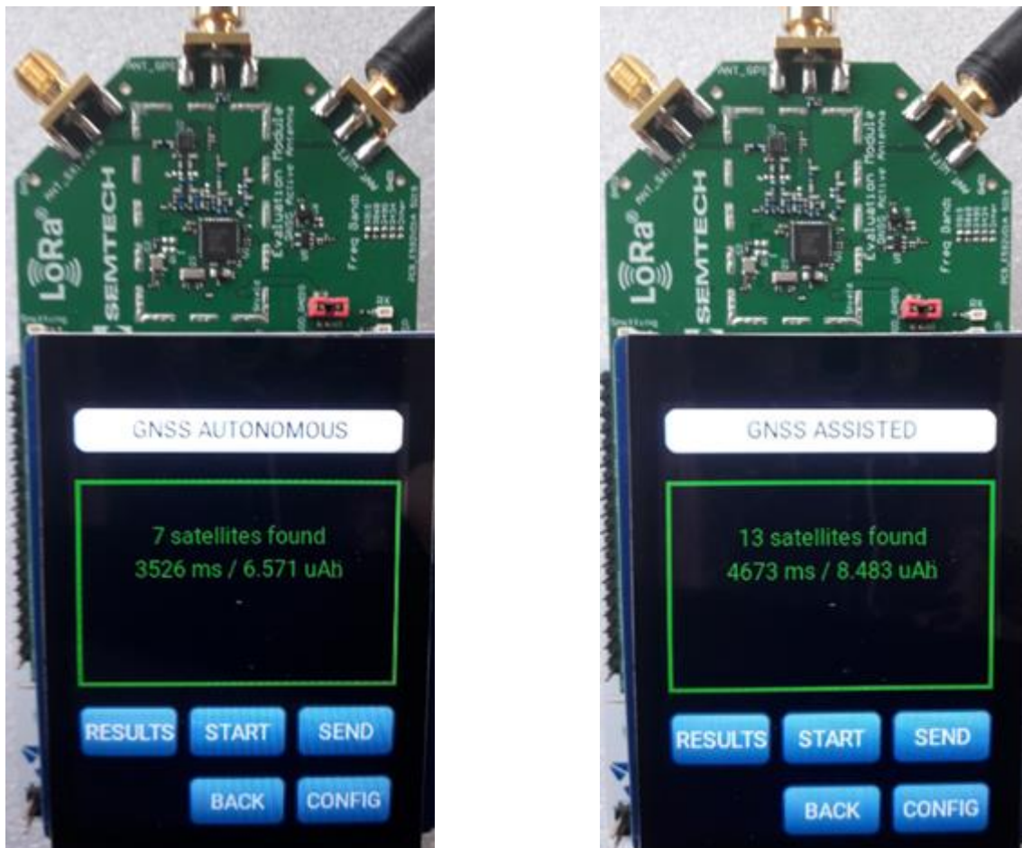
Figure 7: GNSS Autonomous and Assisted Scanning Results
